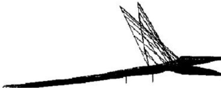
Fig.10(b): Side view of the Bridge showing the deflected structure superimposed onto the original one.
