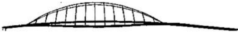
Fig.10(a): Longitudinal view of the Bridge showing the deflected shape (due to working loads) superimposed onto the original structure.
