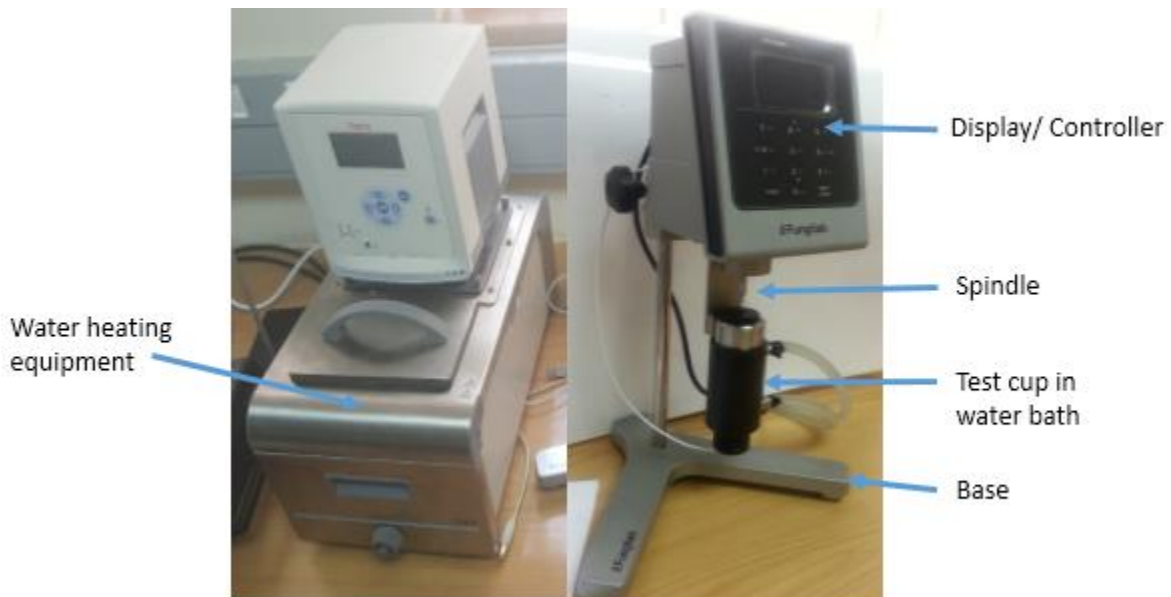
Figure 3-8. Fungilab Premium digital electronic viscometer used for measuring viscosity and Thermo-scientific (Hake AC 150) water heater.
