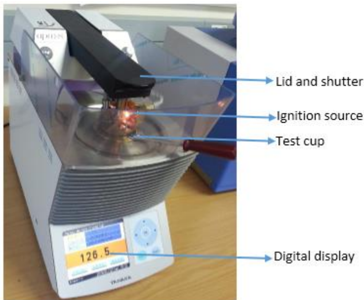
Figure 3-12. Automated Abel closed cup tester used for measuring flash point.
