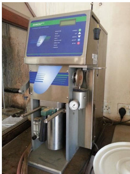
Figure 3-5. Ankom XT15 fat extractor. Source: Sebele Agriculture research lab
