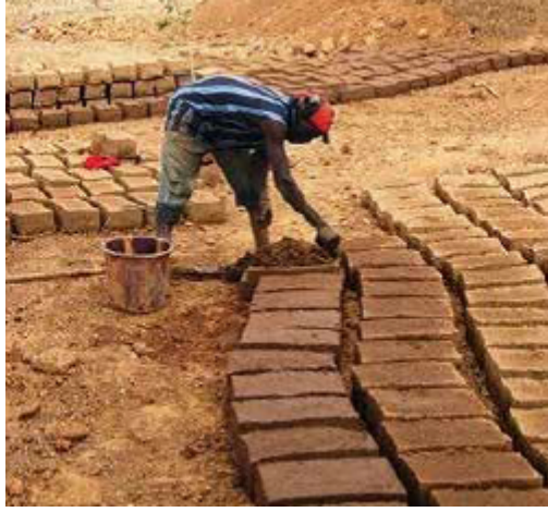
Figure 2.3: Production of adobe bricks.
