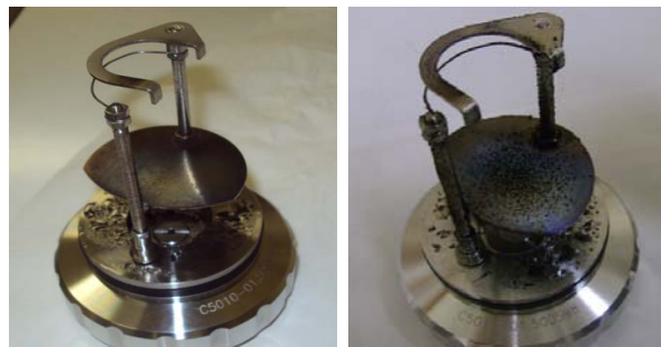
(a) Tylosema biodiesel soot (b) Petroleum diesel soot
